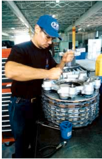
(Top) Joseph Vazquez completing a 727 brake assembly. (Right) Leonard Smith cleaning a wheel casting before the overhaul process begins.
